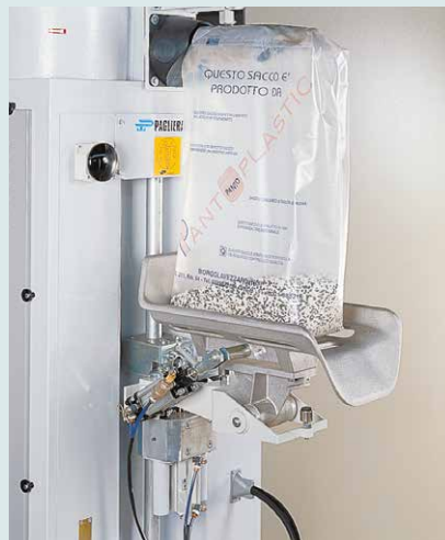
The filling cycle is activated; the bag is suspended so that the weight of the product opens its bottom.
