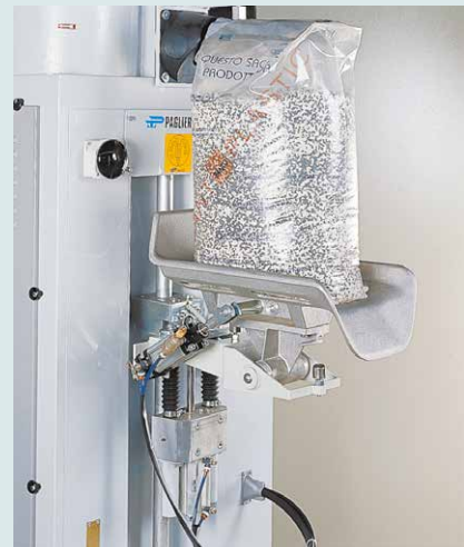
The cradle rises to support the product and start the vibration.
