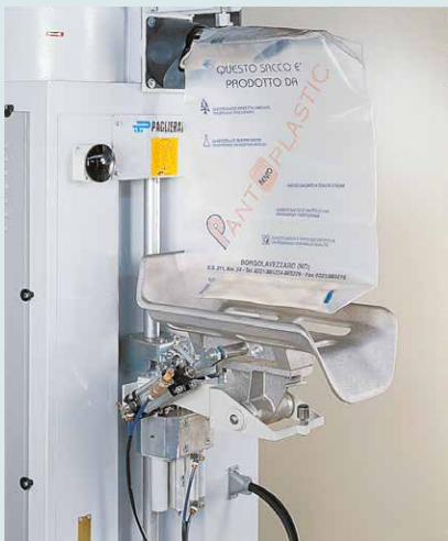
The empty bag is put in place (cradle in low position).
